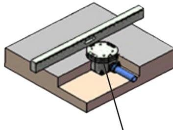
Make sure montage-box is vertical and centered to you. Tighten up montage-box to hole bot tom with 4pcs MS expansion screws, make sure floor tile must be higher than bottom line and lower than middle line of montage-box.
